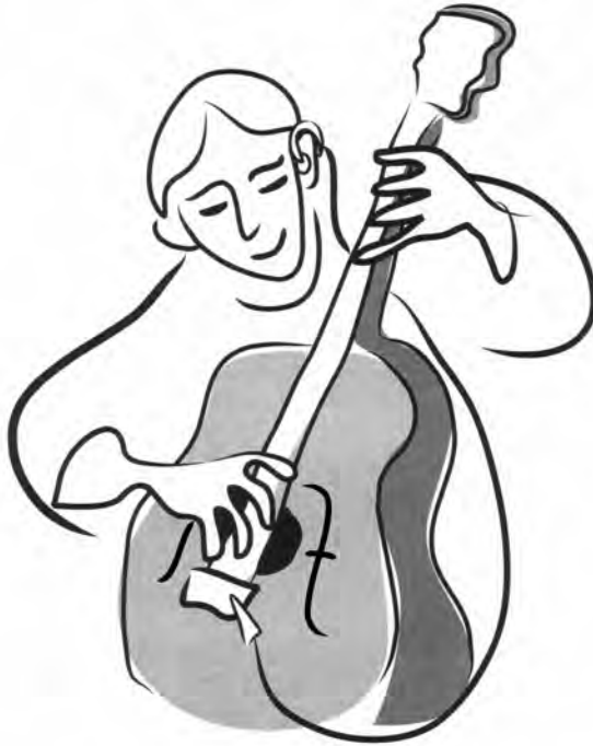
Figure 3-7: An acoustic monitoring device consists of a length of standard hearing aid tubing that joins an earplug (usually a vented/tuned earplug) to a bass instrument. The attachment can be clipped onto the tailpiece, taped to the instrument body, or simply placed in a “f-hole”. It is essentially a stethoscope.
